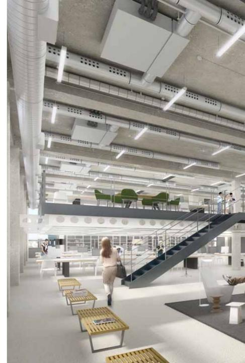
THE PRINCIPLE OF THE WHITE COLLAR FACTORY IS TO OPTIMISE THE CLIMATE CONTROL BENEFITS OF THE BUILDING'S PASSIVE DESIGN (TALL CEILING, WELL INSULATED FACADE, EXPOSED MASS) TO REDUCE THE LEVEL OF MECHANICAL AIR CONDITIONING REQUIRED. THE BUILDING IS NATURALLY VENTILATED AT THE PERIMETER WITH RADIANT SLABS PROVIDING BACKGROUND COOLING AND HEATING.
