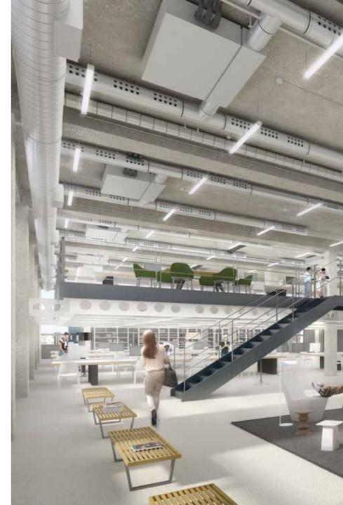
THE PRINCIPLE OF THE WHITE COLLAR FACTORY IS TO OPTIMISE THE CLIMATE CONTROL BENEFITS OF THE BUILDING'S PASSIVE DESIGN (TALL CEILING, WELL INSULATED FAÇADE, EXPOSED MASS) TO REDUCE THE LEVEL OF MECHANICAL AIR CONDITIONING REQUIRED. THE BUILDING IS NATURALLY VENTILATED AT THE PERIMETER WITH RADIANT SLABS PROVIDING BACKGROUND COOLING AND HEATING.
