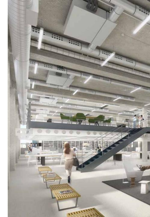
THE PRINCIPLE OF THE WHITE COLLAR FACTORY IS TO OPTIMISE THE CLIMATE CONTROL BENEFITS OF THE BUILDING'S PASSIVE DESIGN (TALL CEILING, WELL INSULATED FACADE, EXPOSED MASS) TO REDUCE THE LEVEL OF MECHANICAL AIR CONDITIONING REQUIRED. THE BUILDING IS NATURALLY VENTILATED AT THE PERIMETER WITH RADIANT SLABS PROVIDING BACKGROUND COOLING AND HEATING.
